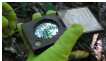
Measuring forest overstory density with Densiometer
